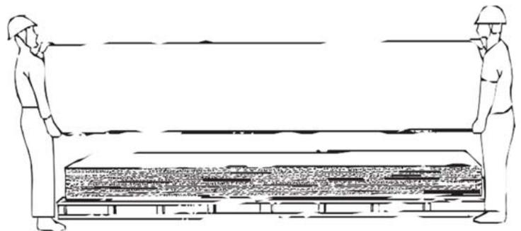
Zintra must be stored in a dry location. It is advised to use a polyethylene sheet which can serve as a draped cover over any stored panels. Panels should be stored indoors in a cool (50-85 degrees F), dry, ventilated area which is out of direct sunlight and away from any heating sources.
